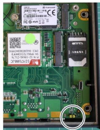
**6** Connect the AC adapter to the Edge AI Box power connector.
